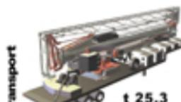
crane and complete ballast on 1 truck
